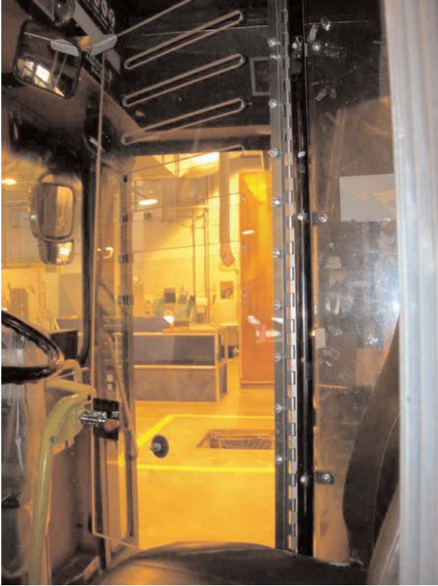
FIGURE 17 Milwaukee County Transit System prototype barrier with slots. (Courtesy: Milwaukee County Transit System.)
