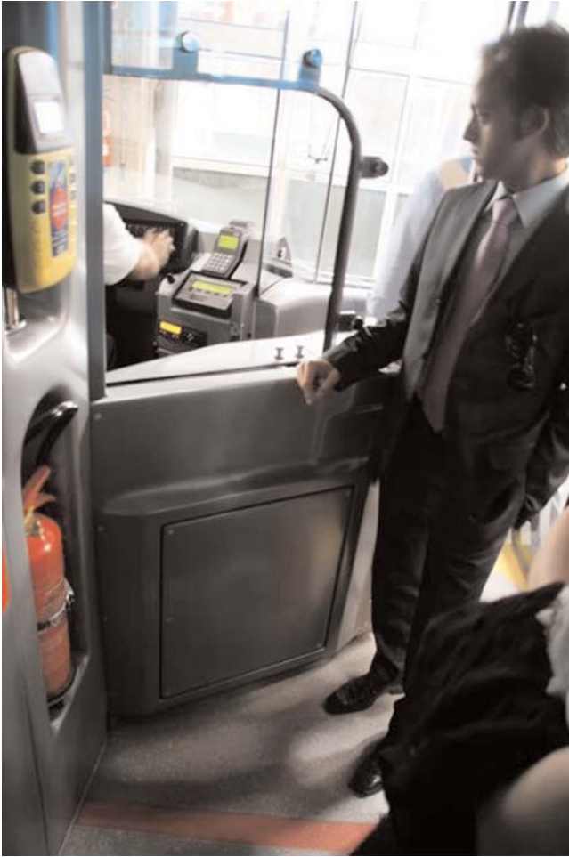
FIGURE 20 Lisbon enclosure, passenger service window open. (Courtesy: Dr. Frank Goldsmith, TWU Local 100.)
