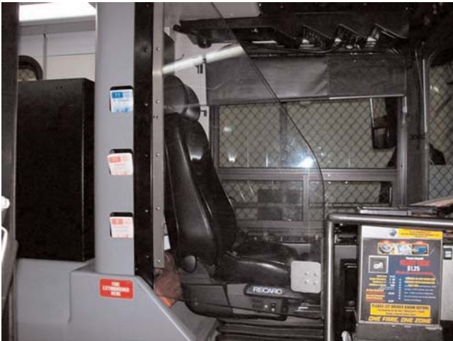
FIGURE 18 Rochester Genesee RTA barrier, closed. (Courtesy: Rochester Genesee Regional Transportation Authority.)
