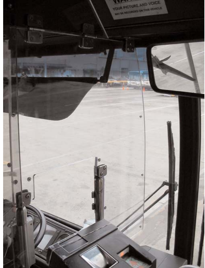
FIGURE 16 SF MUNI barrier, upper portion. (Courtesy: SF MUNI.)
